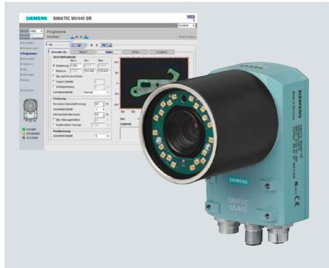
With the "Pat Genius" object recognition license, SIMATIC MV440 can also be used for object recognition (object classification, position detection, counting, etc.) in addition to reading 1D bar codes and 2D matrix codes. In addition, the functionality is possible in combination with text recognition, for example, thus enabling position control of a label and control of the labeling (reading and comparison) of plain text in an image field.
