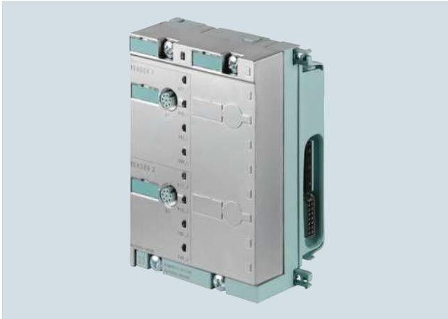
The SIMATIC RF170C is a communication module for connecting the SIMATIC identification systems to the ET 200pro distributed I/O system. The readers (SLGs) of all RFID systems as well as the MV400 code-reading systems can be operated on the SIMATIC RF170C.
