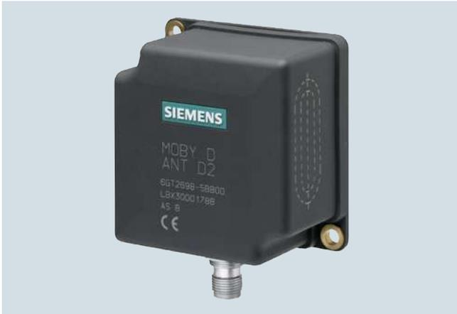
The ANT D2 antenna is designed for transponders that pass the antenna at the side. This antenna is specially designed for high speeds, e.g. in overhead conveyors, assembly lines, production and order picking. It can be mounted directly onto metal surfaces.
