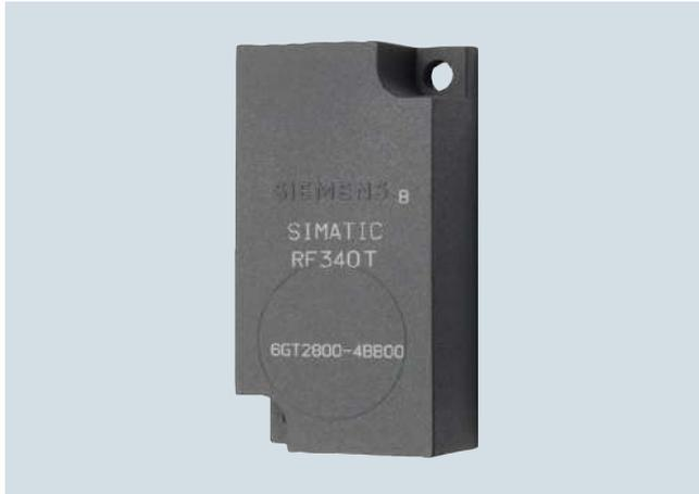
Universal transponder (8 KB FRAM + 24 byte EEPROM + 4 byte serial number), particularly suitable for small workpiece carriers. For mounting directly onto metal.
