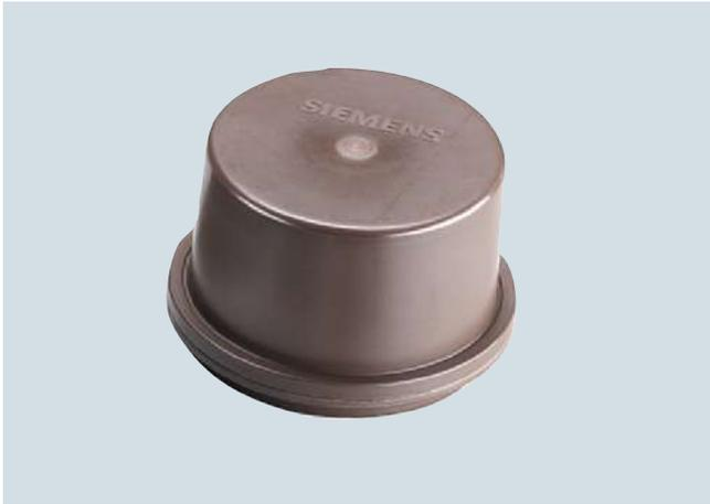
Heat-resistant, rugged transponder for use in paint shops (auto-mobile industry, primer/top coat) or applications with similar temperature requirements, memory capacity 32 KB RAM, temperature range -25 °C to +85 °C, up to +220 °C cyclically, IP68 degree of protection, enclosure dimensions (mm) Ø 114 x 83.
