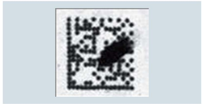
Damaged surface of the marking or part
