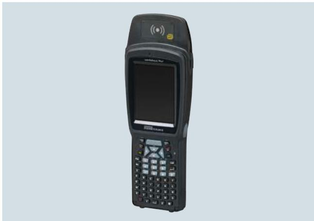
SIMATIC RF680M is a powerful, mobile RFID reader for applications in the field of production logistics, warehouse management, inventories and service. The device is also an important tool for commissioning and testing of RFID systems. Thanks to the high transmit power, the RFID transponders can even be reliably detected at large distances.
