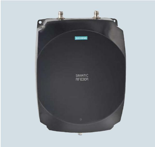
The UHF RFID reader SIMATIC RF630R has been specially designed for the requirements in production. The reader can be used with one or two external antennas (SIMATIC RF620A/640A/642A/660A). The device is integrated into automation systems via the RS422 system interface. Connection to PROFIBUS, PROFINET, and Industrial Ethernet or directly to SIMATIC S7-300 is supported (via communication modules SIMATIC RF170C/180C/182C or ASM 456/475).
